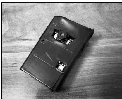
Fig. 6. Custom built frame for camera. In our CCTV surveillance hardware setup, as shown in figure 6, simplifies installation by combining power supply and data transmission in one cable. The entire system is securely housed, ensuring the reliability of our single-camera CCTV surveillance solution
